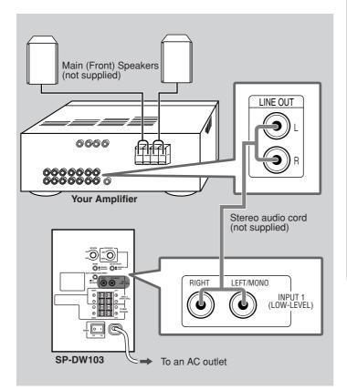
If your amplifier has only a monaural line output (MONO) jack, connect it to the LEFT/MONO jack of the INPUT 1 (LOW-LEVEL) terminal (see **Connecting Method** A).
