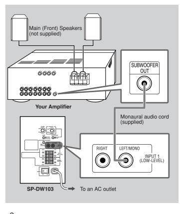
When using **Connecting Method** A, no signal comes out of the TO MAIN SPEAKERS terminal.
